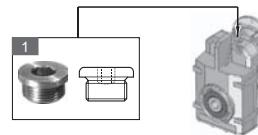
All the gearboxes are furnished with a solo cork of unloaded / load of the type 1.
